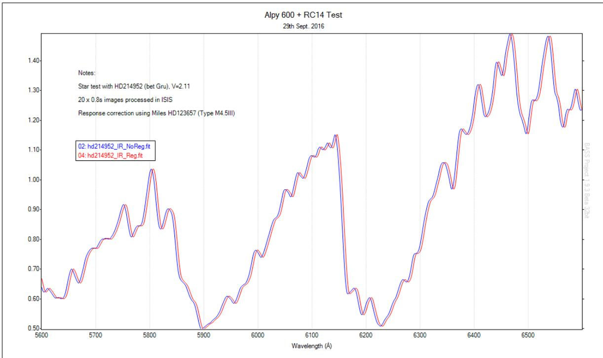
Figure 16: A comparison of spectra with wavelength registration disabled (blue) and enabled (red) of the Type-M star HD214952. The red profile shows an unexplained shift of approximately  $2.5\text{\AA}$ .
