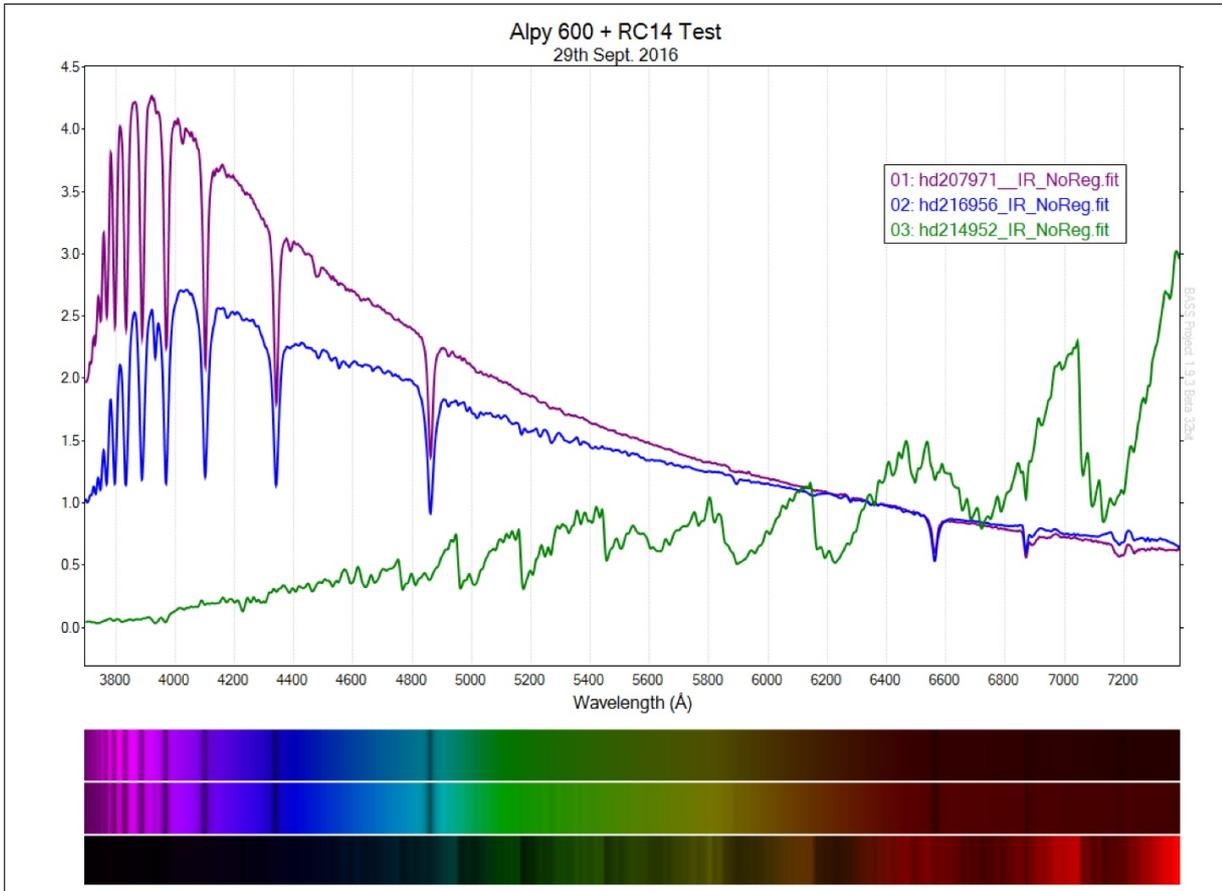
Figure 14: Three bright star test profiles and their synthetically generated spectral strips.
