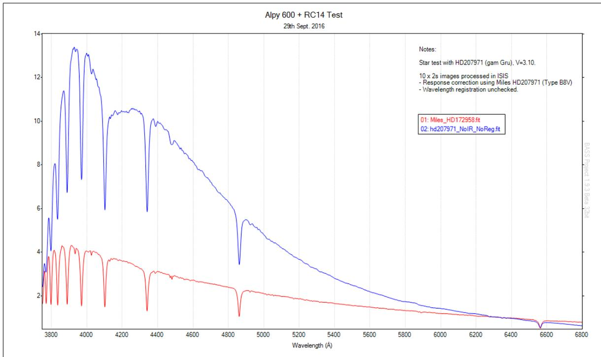
Figure 2: The wavelength calibrated spectrum of HD207971 **without** instrument response correction applied compared to a Miles B8V standard (both spectra have been scaled to unity at 6355Å).
