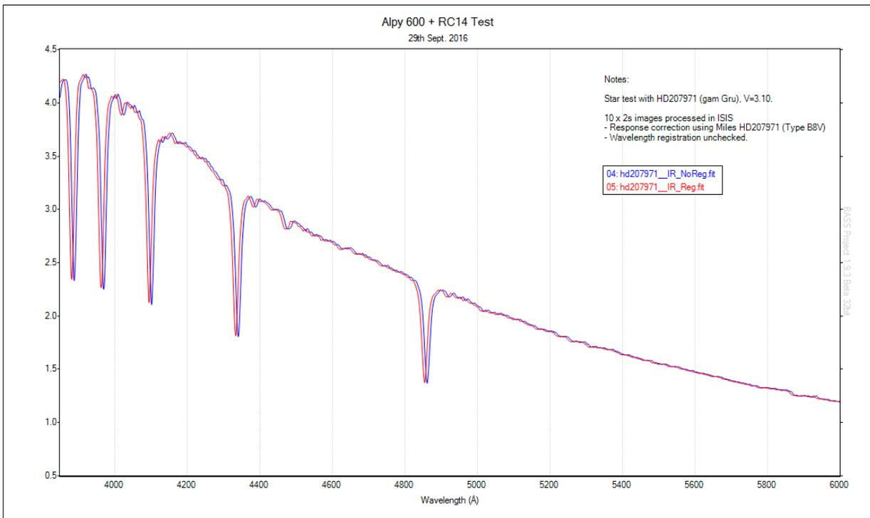
Figure 15: A comparison of spectra with wavelength registration disabled (blue) and enabled (red). The red profile exhibits an unexplained shift of approximately  $5\text{\AA}$ .
