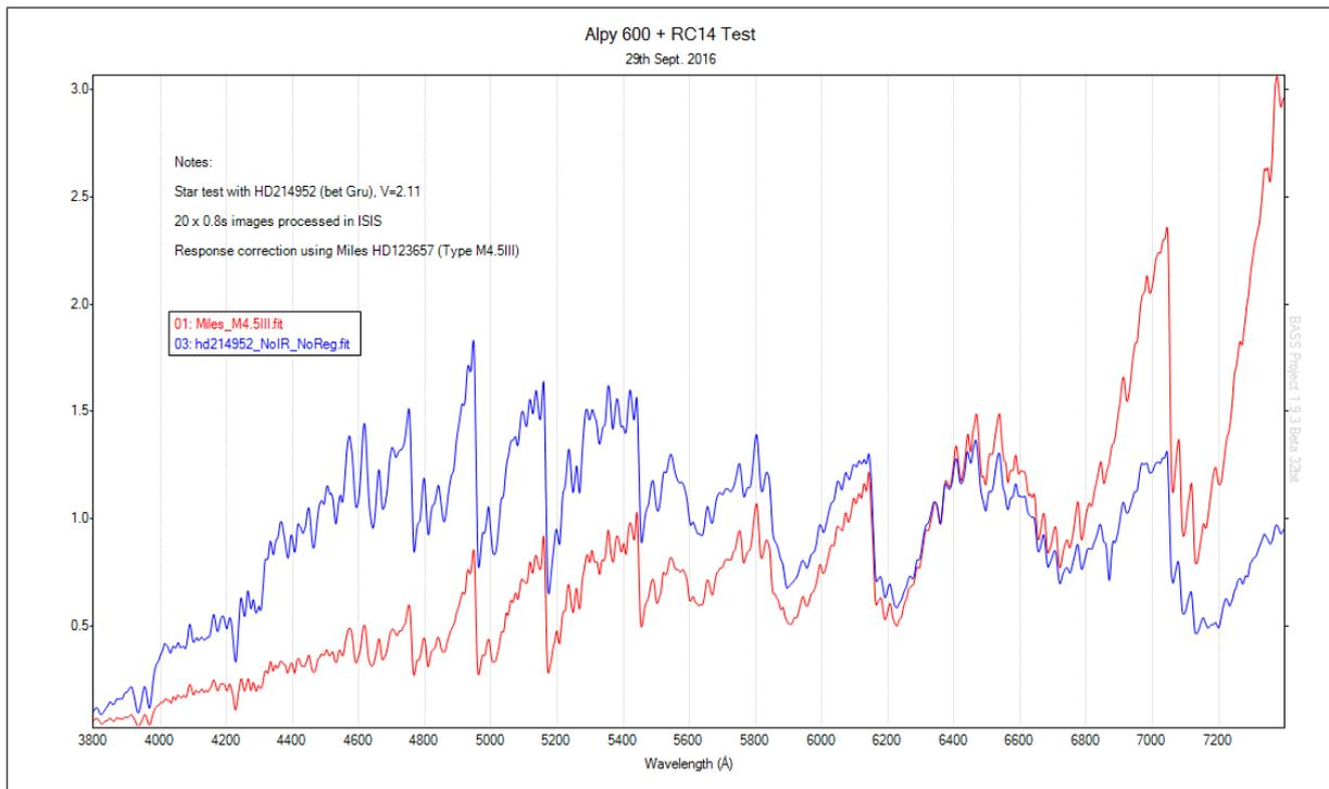
Figure 8: The wavelength calibrated spectrum of HD214952 **without** instrument response correction applied compared to a Miles M4.5III standard (both spectra have been scaled to unity at  $6355\text{\AA}$ ).
