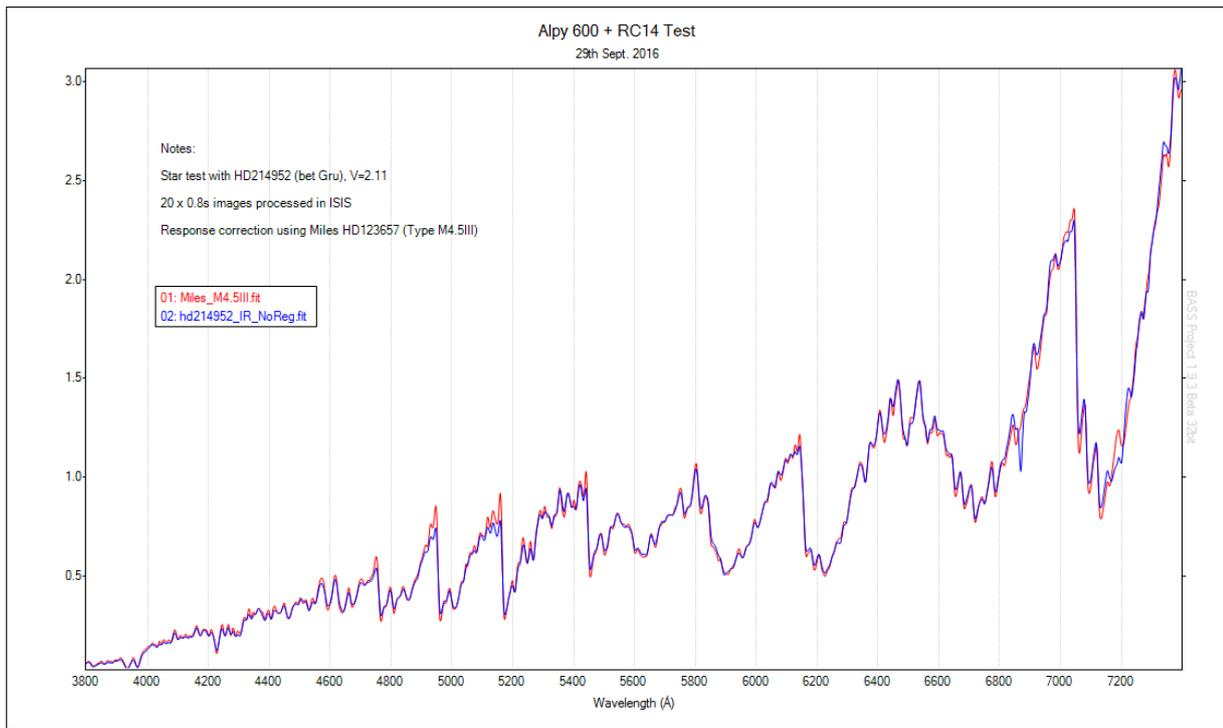
Figure 9: The calibrated and instrument response corrected spectrum. The acquired spectrum (blue) compared to a Miles M4.5III standard (Red) shows excellent alignment to wavelength and temperature profile.
