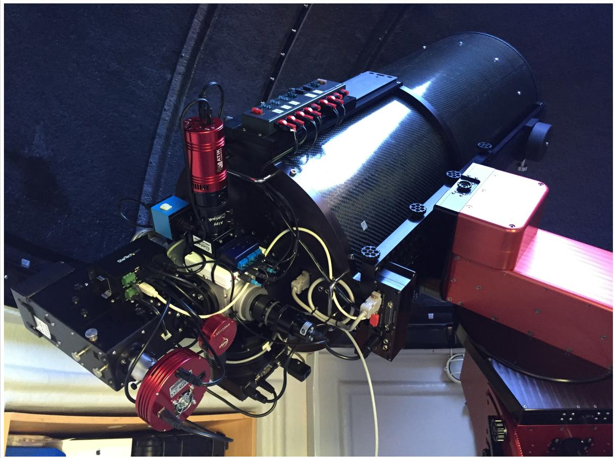
Figure 1: The RC14C telescope's optical manifold which allows manual selection of instruments. The Alpy 600 is located at the 3 o'clock position and includes a calibration unit and a video feed for target positioning on the slit. The image train also includes a Lhires III spectrograph (rear most instrument) and a photometric CCD camera (barely visible at the 9 o'clock position).
