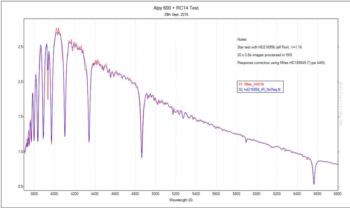
Figure 10: The calibrated and instrument response corrected spectrum of HD216956. The acquired spectrum (blue) compared to a Miles A4III standard (Red) shows excellent alignment to wavelength and temperature profile.
